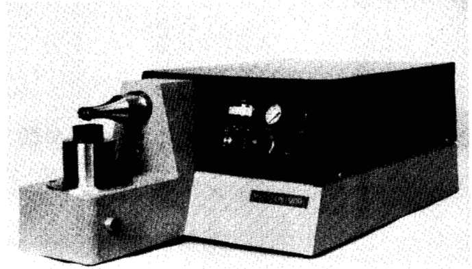
Fig. 10. 1200 W, 20 kHz ultrasonic metal welder. Lap welds are produced by ultrasonic shear at the interface.
